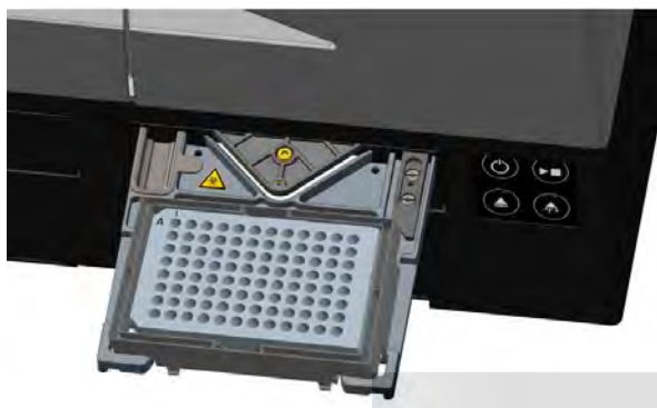
Figure 97: Microplate on the plate carrier with the A1 well in the upper left-hand corner
