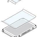
5. While applying firm downward pressure, move the applicator slowly across the film, both horizontally and vertically, to ensure good contact between the film and the entire surface of the reaction plate.
