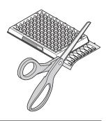
**IMPORTANT!** Completely remove the fill reservoirs from the array card so that the edge is free of residual plastic. The plastic from the fill reservoirs that extends beyond the edge of the card can prevent the array card from seating properly on the sample block and can affect amplification.
