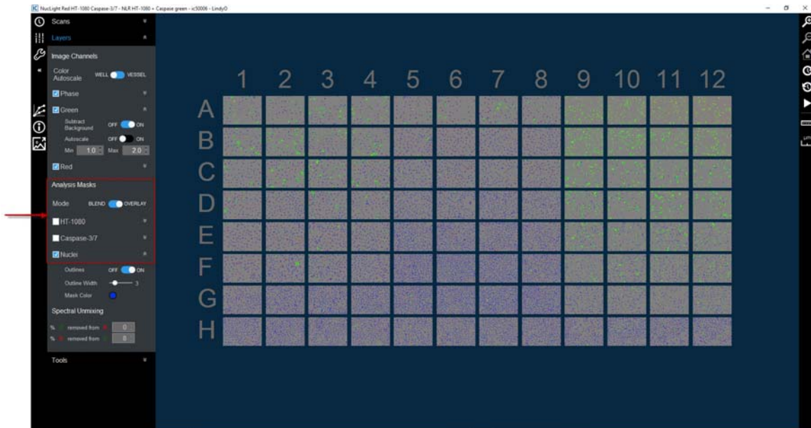
Figure 2-1: Vessel View with the associated analysis window, toggling image masks on and off
