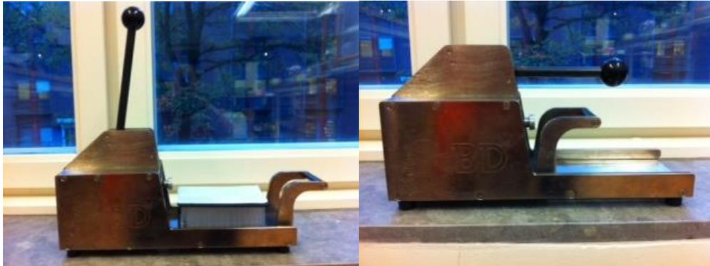
*Figure 1. Demonstrate plate sealer usage for optimal sealing of Greiner deep well blocks. Use two rubber spacers on top of the Deep Well Block to be sealed with the nice rubber side facing the aluminium foil (left). Slide the Deep Well Block with rubber spacers into the plate sealer and adjust the rubber spacer position on top of the Deep Well Block and press the handle (right). Wait for 30 seconds – done!*
